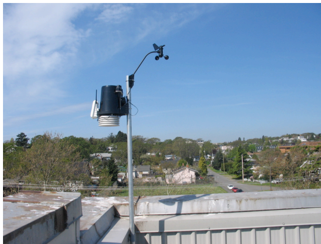
Figure 2. Photograph of the Davis Vantage Pro2 Plus weather station installed on top of Oaklands Elementary school in Greater Victoria School District 61.
